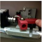
Push the red release levers. This will allow you to pull the drawer open from the front.
